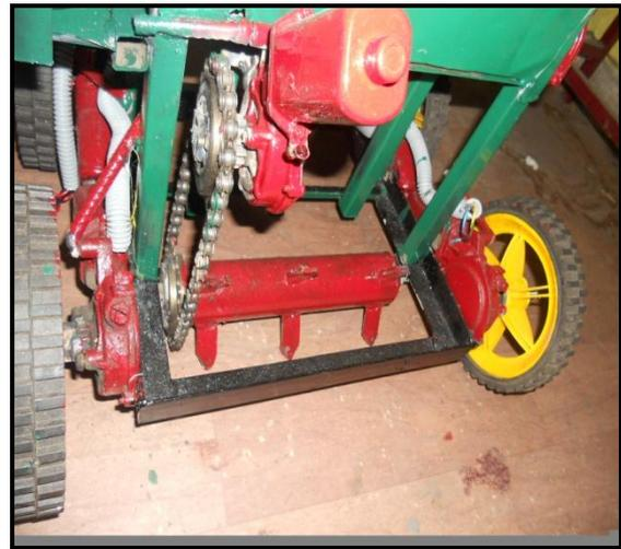
**Figure 2.4.2:** Digging Tool Arrangement
